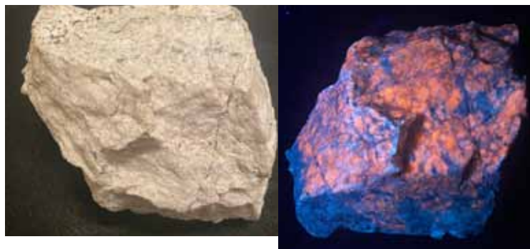
Scapolite from near Secesh Summit under visible light (left) and LW UV (right).
